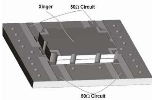
**Figure 3: Component Placement**
