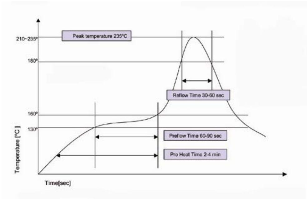
Figure 5 – Low Temperature Eutectic Solder ( 63/37) Reflow Thermal Profile
